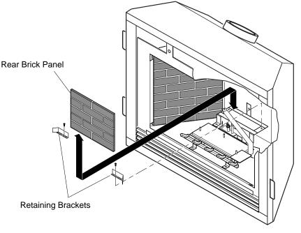
Figure 45- Installing Rear Brick Panel and Retainer Brackets
